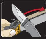
Hold the handle so the leather strop is facing up. Place the side of the blade on the stropping Guide with the cutting edge facing down and away from the leather.
